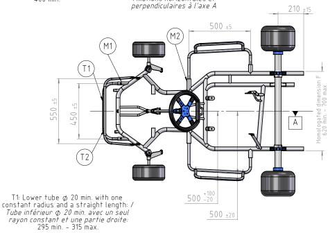
T2: Upper tube  $\phi$  16 min. with one constant radius and a straight length: /
